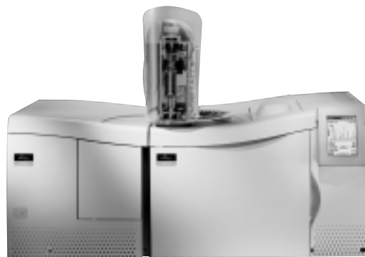
The Clarus 500 GC/MS system includes a quadrupole MS with the mass range of 1-1200 daltons, providing very fast scan speed, up to 60 scans/second, and permits Selected Ion Full Ion (SIFT™) monitoring in the same run, simultaneously acquiring data in full scan together with Selected Ion Monitoring (SIM).
