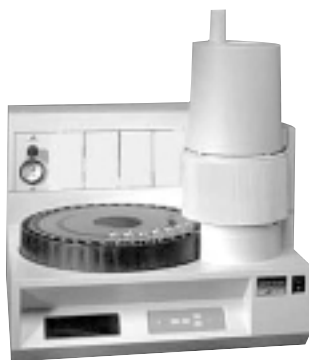
The HS 40XL Automatic Headspace Sampler was the seventh generation of headspace samplers. On the left is the carousel where the samples are placed. The tower on the right side is where the vials are heated and the volatiles transferred to the gas chromatograph.
