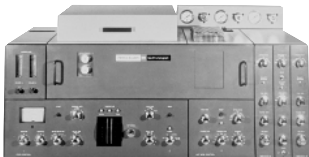
The Model 900 Gas Chromatograph . The column oven opens on the top left, with two FIDs in the wire cage to its right. Behind this are the controls for three gases, the carrier gas (helium), as well as hydrogen and air for the FIDs. The dual injection port is left of the name plate. The various knobs represent temperature controls and controls for the detector electronics.
