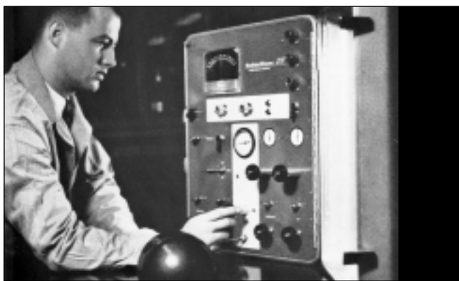
The Model 213 Hydrocarbon Analyzer . It was a portable unit, permitting the analysis of atmospheric samples for the total organics content, with help of a flame-ionization detector.
