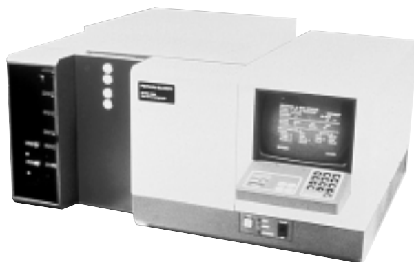
The Sigma 2000 was an electronically controlled gas chromatograph with a built-in display of the method and the actual conditions. Shown in the middle are the four injection ports that permitted the installation of four columns simultaneously.
