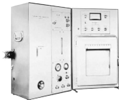
The Model 154-D . In this unit, the amplifier of the flame-ionization detector was incorporated in the upper part of the recorder cabinet (right). The rotary-type gas sampling valve, originally introduced with the Model 154-B, is mounted on the left side of the instrument cabinet.
