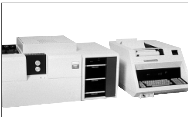
The microprocessor-controlled Sigma 1 Gas Chromatograph is shown with its data system on the right.
