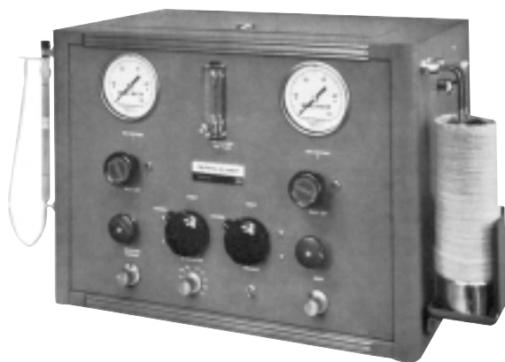
The Perkin-Elmer-Shell Model 212 Sorptometer was developed for the determination of the surface area of solids according to the BET method, using a GC-type measurement. The sample holder was placed in the Dewar flask on the right where adsorption took place at liquid-nitrogen temperature.
