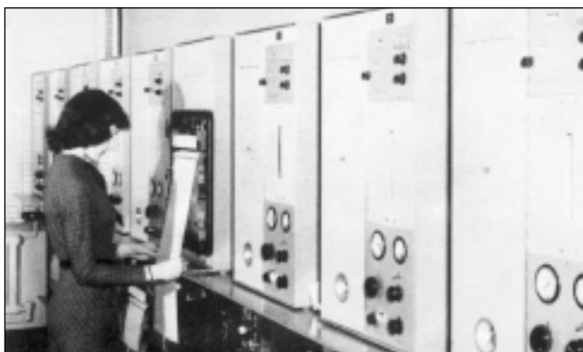
Routine gas chromatography laboratory at Esso R&D Co., in early 1958. This room contained at that time eight Model 154 Gas Chromatographs . Except for the unit attended by the operator, the potentiometric recorders were placed directly under each chromatograph. (From W.A. Dietz, Instrument News , Spring 1958 edition.)
