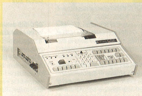
The Chromatopac C-R1A electronic data system had a built-in printer-plotter and was introduced in 1978.
