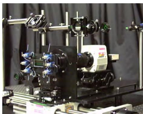
Fig.2 Photograph of the capillary isoelectric focusing system with fluorescence-imaging detection.
