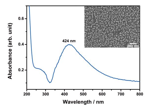
Fig. S2 UV-Vis extinction spectrum of Ag NPs and the SEM image of the assembled Ag NPs film (inset).
